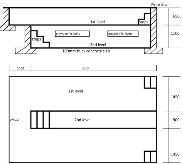
50 x 50 x 3 Angle iron edge rails around pit built into corner Plastic underlay to prevent water seepage into pit 220 volt plug point at front of pit to supply equipment Air point inside of pit for pneumatic tools
